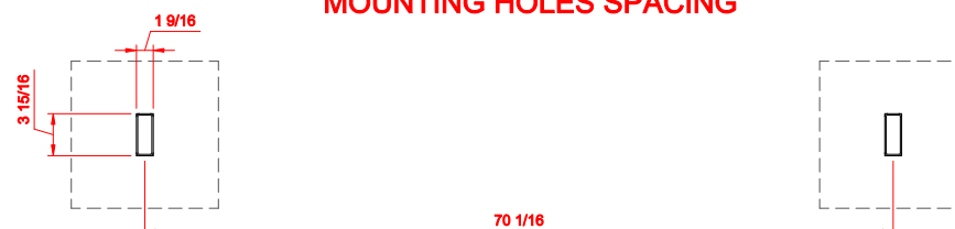
MOUNTING HOLES SPACING
